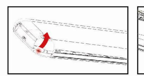
2. Remove the battery if it is in. Locate the SIM card slot and insert the proper SIM card into the proper slot. For more information on SIM card installation, check out the included SIM Card & Micro SD Card
