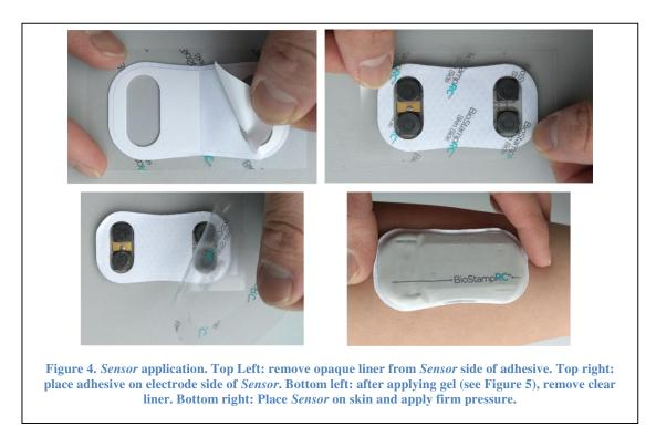
The BioStampRC system comes with a tube of conductive gel for use in facilitating electrode measurements. The use of this gel is essential for obtaining the highest quality electrical signals from the BioStampRC system. Apply a small amount to each electrode as shown in Figure 5. Only a thin coating is needed; wipe off any excess gel. Excessive use of gel may adversely affect *Sensor* adhesion.
