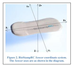
The BioStampRC Sensor can be placed in various body locations, and multiple Sensors can be placed on a single person. Once configured using the Investigator App, the Sensor operates independently, storing data in
