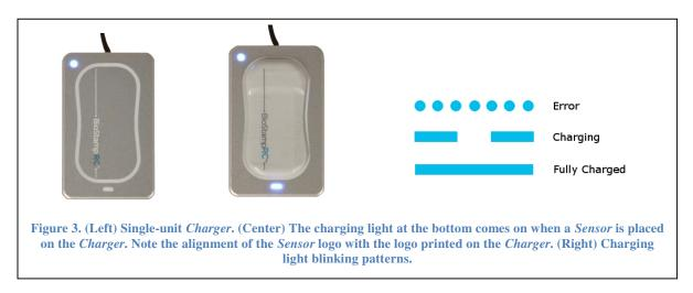
When the *Charger* is plugged into a wall outlet, the power light in the upper left corner comes on (Figure 3, Left). The charging light near the bottom of the charger should be off. If this light is blinking rapidly (Figure 3, Right), the charger experienced an error and must be restarted.
