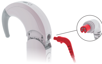
Fig. 27 Plugging the coil cable into control unit
