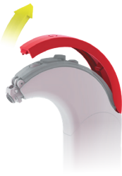
Fig. 35 Removing the microphone cover
