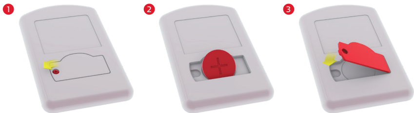
Fig. 44 Changing the battery of your FineTuner
