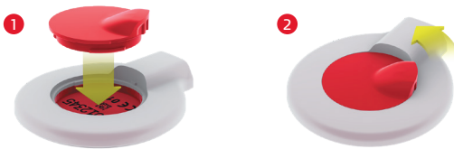
Fig. 22 Inserting the magnet
