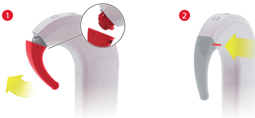
Fig. 33 Attaching the earhook
