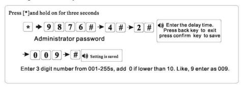
5.63 Exit delay setting: the period from user arm to the system armed successfully. This is for user's convenience to exit after arm operation.(default value is 10s)
