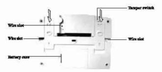
2.Mark and drill holes in mounting surface, fasten the bracket to the mounting surface with screws.
