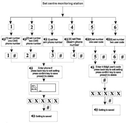
The user code in the CMS setting which is identification code in the CMS. And the user code in transfer alarm setting is user, identification code between same model panel
