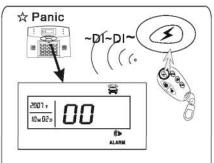
Press the panic button on remoter, or press "help/bypass" key on panel for 3 seconds, and 10 seconds later the panel will dial the preset phone number. And you can disarm to cancel alarm.
