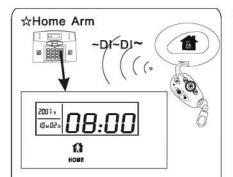
Press the key for home arm on the remote or "HOME" key on the keypad, the panel will give voice to tell system is enter home arming. And it display home arm icon on the LCD screen.
