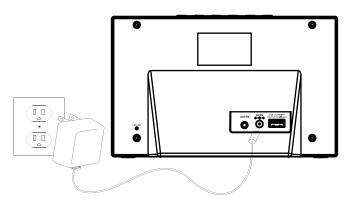
Plug the included AC/DC power adapter (100-240V 50/60 Hz 5V/1A) into the DC Jack on the rear of the unit and the other end is plugged into the wall outlet.
