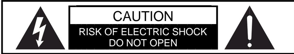
CAUTION: TO REDUCE THE ELECTRIC SHOCK, DO NOT REMOVE THE COVER (OR BACK). NO USER SERVICEABLE PART INSIDE, REFER SERVICING TO QUALIFIED SERVICE PERSONNEL.
