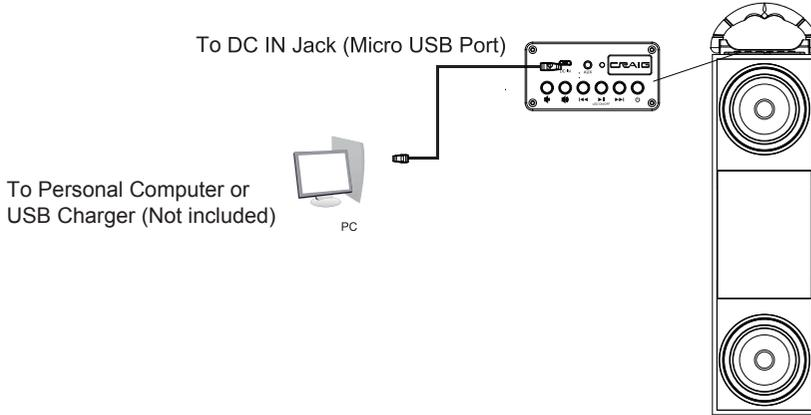
3. During charging, the Red Charging Indicator on the top of unit will illuminate. When finished, it will turn off.
