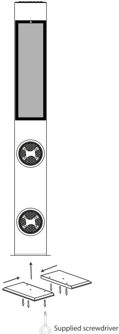
Assembly the two wooden bases to the bottom of unit by the supplied assembly screws and screwdriver as the illustrated above.
