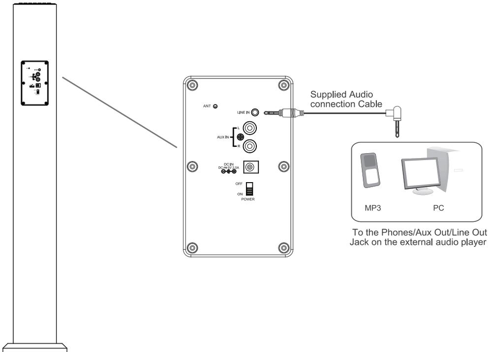
3. Power on the unit and enter to LINE IN mode as the instructed earlier. The color of the indicator on the top of unit will turns to Purple.
