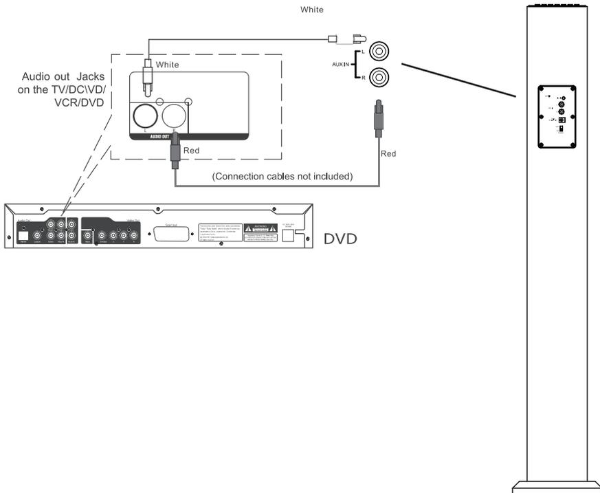
3. Power on the unit and enter to AUX IN mode as the instructed earlier. The color of the indicator on the top of unit will turns to Green.
