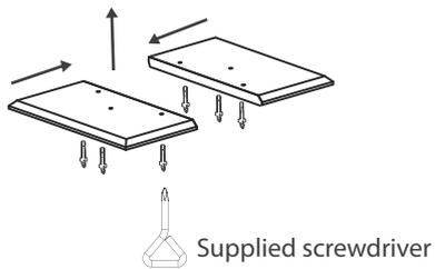
Assembly the two wooden bases to the bottom of unit by the supplied assembly screws and screwdriver as the illustrated above.
