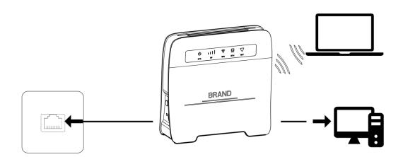
Scenario 3: Data service from Ethernet cord and VOLTE voice using a SIM card
