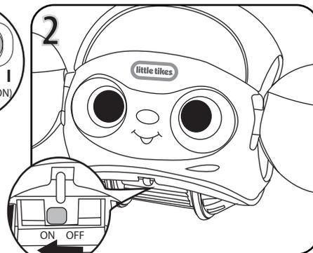
Move the switch under the RC car from OFF to ON. The light on the center button of the remote will remain solid, indicating the remote and RC car are paired.
