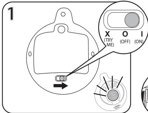
Move the switch on the back of the controller to the ON (I) position. The light on the center button of the remote will flash.
