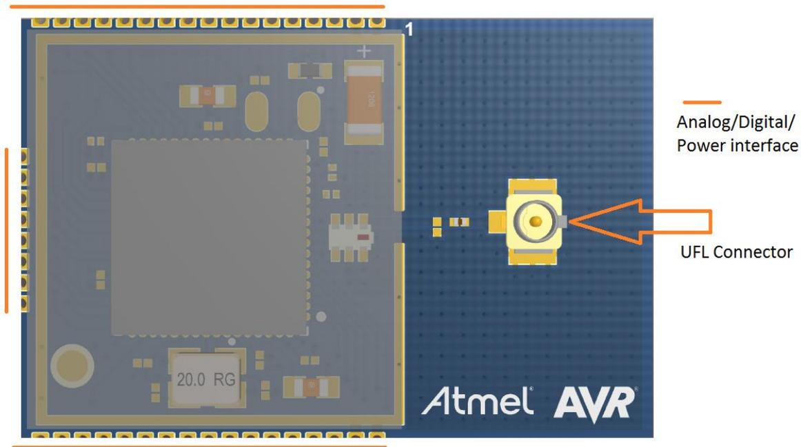
This ZigBit module contains the Atmel ATmega256RFR2 Microcontroller and a 2.4GHz ISM band Transceiver for ZigBee and IEEE 802.15.4 [1]. The module features 256KB In-System Self-Programmable flash memory, 32KB SRAM and 8KB EEPROM.
