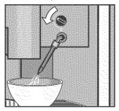
■ Place a 1 liter container below the steam nozzle and turn the steam selector counterclockwise.
