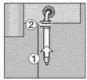
■ Push the sleeve onto the steam nozzle. (1), and tighten the screw, (2).
