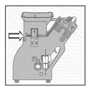
The basic position shown above is reset and the brew unit can be set back into the machine.
