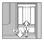
■ Lift the water tank up and out of the appliance.
