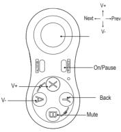
Mini plus is with inner rechargeable lithium battery, please insert 5V USB port to charge, then charging Red LED will be on. And when power is full, Charging Red LED will be off.
