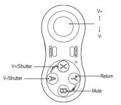
In key mode, press the SELECT button and change Joystick mode into Mouse mode(only on the android platform), Mainly for watching VR Movie.
