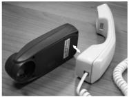
Place the microphone of the telephone (the microphone is near the cable) near to the spirobank II as shown in the figure, with the phone receiver (beneath the device's ID label). The hole should be close to (2 to 5 cm) the microphone's hole positioned on the receiver.
