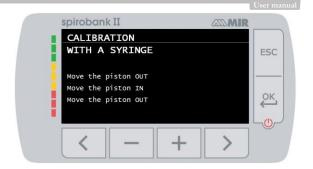
The screen requires to insert the volume of the syringe in use; SPIROBANK II so calculates the correction percentage between the reference and the calculated value. It can be possible to change the syringe volume using and the then press . At this point two new correction values are shown. Press to apply these correction, otherwise press ESC to set the factory calibration values (0%).
