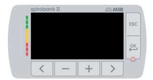
The first screen shows the manufacturer logo, information of date and hour set on the device. If no key are touched, after a few seconds the device shows the main screen.
