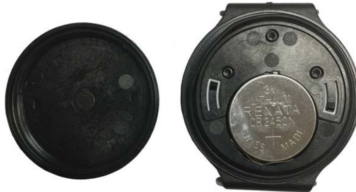
Figure 8: MBD-2 Battery Cover Removed
