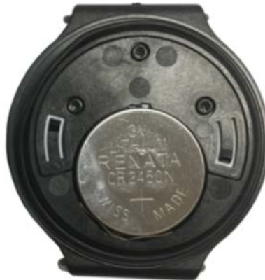
Figure 11: MBD-2 Correctly Installed Battery Position
