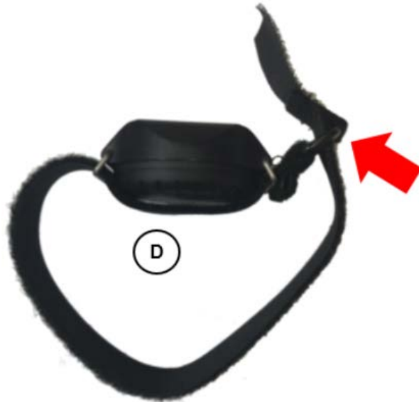
Figure 6: Preparing the Wrist Strap
