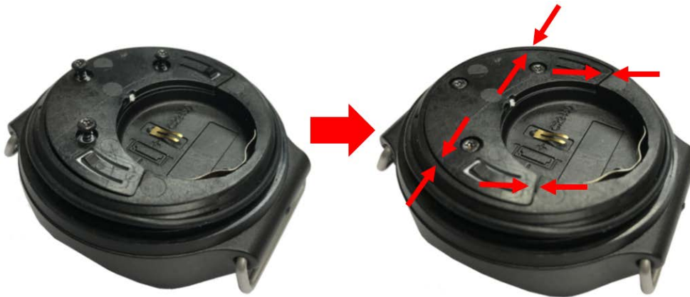
Figure 19: Installing the Internal Battery Cover
