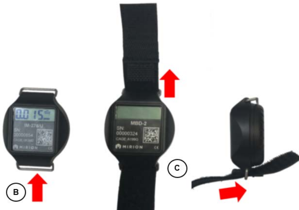
Figure 5: Wrist Strap Orientation and Assembly
