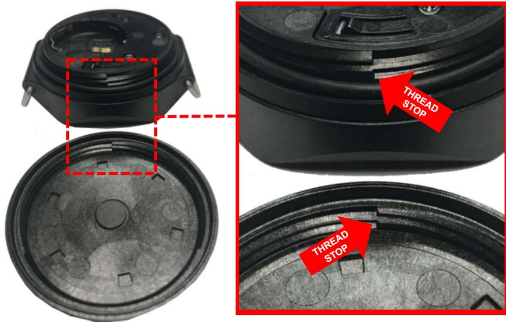
Figure 12: MBD-2 and Main Battery Cover Thread Stops
