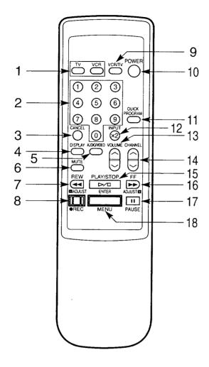
TV and VCR buttons (TV, VCR) In addition to operating your VCR, your VCR remote control can be used to operate most of the functions of many brands of televisions. Press the VCR button to use the remote to operate the VCR. After setting up your remote for your particular brand of television, press the TV button to use the remote to operate your television. See your TV owner's guide for more information about operating your TV.
