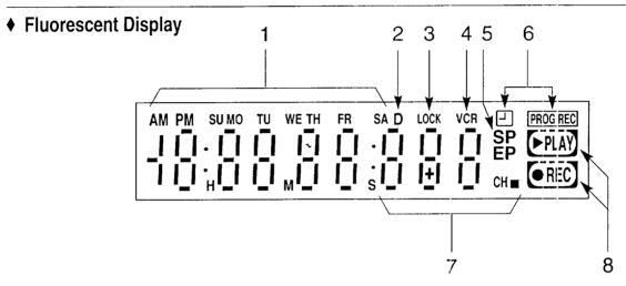
(1) **counter/present time/remaining display** This area displays: the current time; a time counter showing how long the tape has run; the amount of time remaining on the tape; or the contents of a programmed recording when you are programming your VCR.
