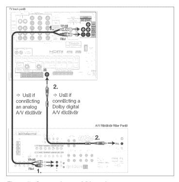
Figure 7. Connecting an A/V receiver
