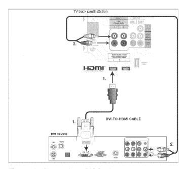
Figure 12. Connecting a DVI Device
