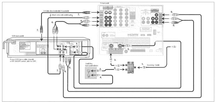
Figure 6. Connecting a VCR to a Cable Box
