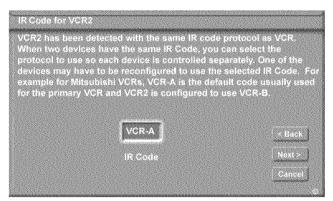
Figure 23. IR Code for [Device] screen
