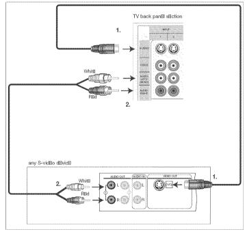
Figure 8. Connecting a Satellite Receiver with S-Video
