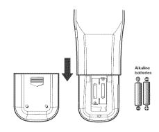
Operation: Installing the Batteries
