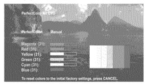
Individual sliders for each color will be displayed. Highlighted text will show which slider you are adjusting. Each TV input or device has a memory for PerfectColor. While using the PerfectColor option, you may reset the colors to the default settings, by pressing CANCEL.
