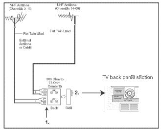
Figure 4. Connecting separate UHF and VHF Antennas
