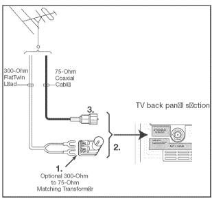
Figure 3. Connecting a Single Antenna
