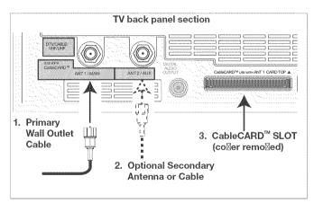
Figure 1. Wall Outlet Cable
