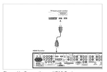
Figure 11. Connecting an HDMI Device
