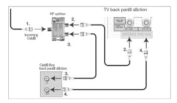
Figure 2. Connecting a Cable Box
