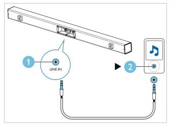
1 Using a 3.5mm stereo audio cable, connect the LINE IN connector on your SoundBar to the LINE connector on the TV or other device.
