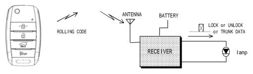
\* Through the use of lamp, operating state is displayed by lamp.
