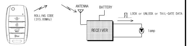
\* Through the use of lamp, operating state is displayed by lamp.
