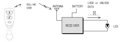
\* Through the use of lamp, operating state is displayed by lamp.
