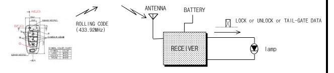
\* Through the use of lamp, operating state is displayed by lamp.
