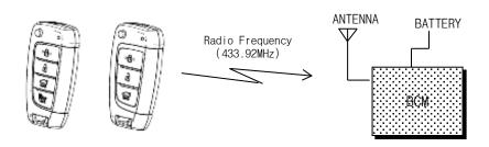
① if press button on the transmitter, RF signal is transmitted and turns on the LED
