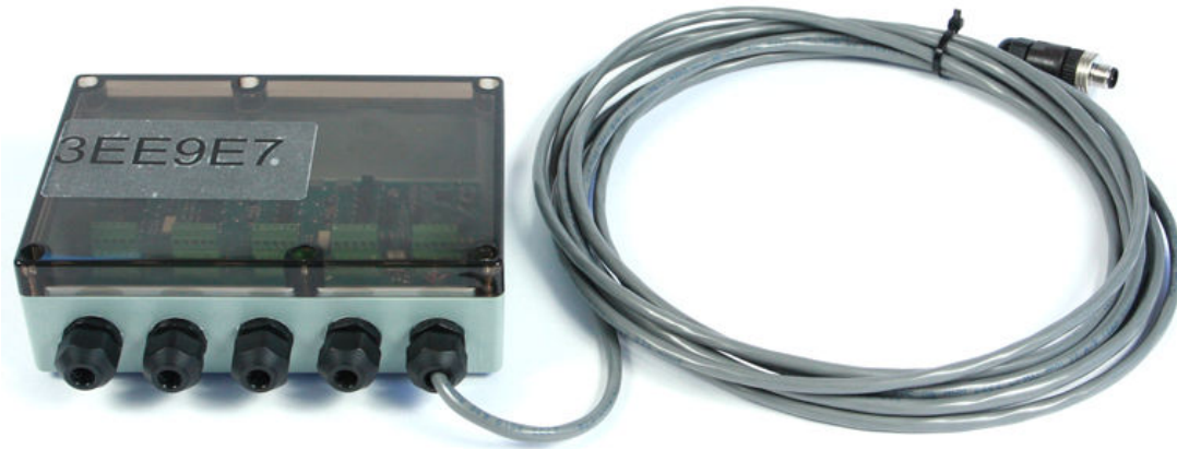
Figure 13: GPIO Unit with RS-485 Cable
