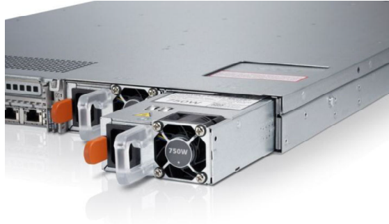
Figure 20: Redundant Power Supplies
