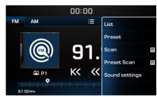
Starting from the current frequency, frequencies with superior reception are scanned for 3 seconds and the previous frequency is restored.
