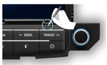
Press and hold the RESET key for about 1 second. (The use of a clip or pin is recommended when resetting the system.)
