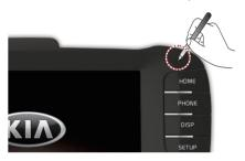
Press and hold the RESET key for about 1 second. (The use of a clip or pin is recommended when resetting the system.)
