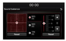
Press the Reset to restore sound to the center position.
