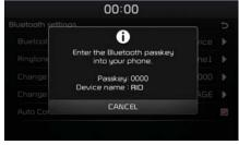
From the Bluetooth® device, search for the car name and pair the device. When searching from the Bluetooth® device, the car name is RIO and the default passkey is '0000'.
