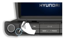
Press the reset hole using a clip or pin.
