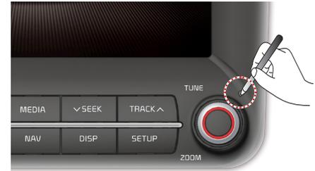
Press and hold the RESET key for about 1 second. (The use of a clip or pin is recommended when resetting the system.)
