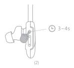
Shutdown state , Long press Power button for "3~4S", enter pairing mode directly.
