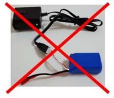
▶ It will reduce the life of battery if no charge when the battery no power or forgot to ap art the connector and charge port of the battery.
