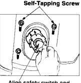
Align safety switch and turn clockwise to secure
