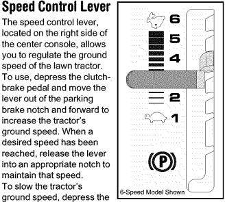
clutch-brake pedal and move the speed control lever rearward and release it into a notch.
