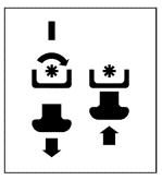
**NOTE**: The PTO (Blade Engage) knob **must** be in the disengaged (OFF) position when starting the engine, when traveling in reverse and if the operator leaves the seat.
