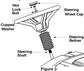
**NOTE:** If the openings on each end of the steering bellow are of two sizes, the smaller end goes down against the dash of the tractor.
