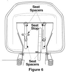
**NOTE:** If the seat was shipped in a box, line up plastic seat spacers with the slots in seat pivot bracket and slide seat in until front seat spacer engages seat stop.
