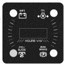
**NOTE:** The hour meter is activated whenever the ignition switch is turned to the "ON" position. Keep a record of the actual hours of operation to assure all maintenance procedures are completed according to the instructions in this manual and the engine manual.
