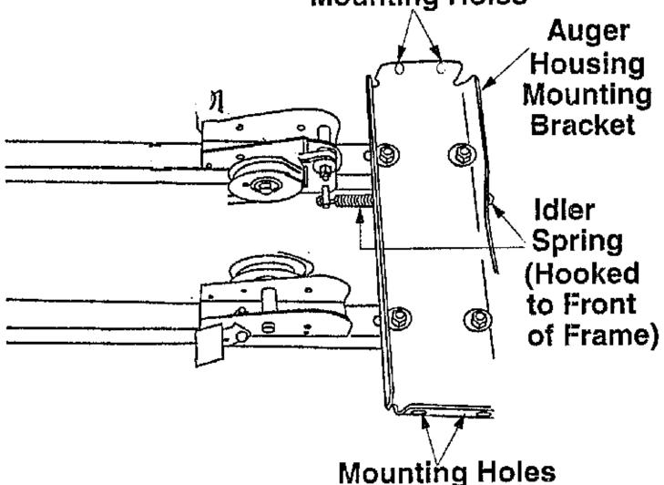
2. Lower auger housing down onto mounting bracket. Align four holes and secure with four hex bolts and lock washers. See Figure 2.
