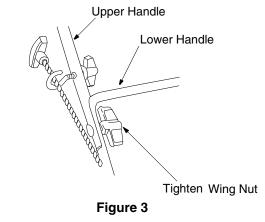
**NOTE:** Make sure to route the cables outside the lower handle. Also do not crimp the cables while lifting the handle up.
