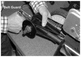
Figure 20 Remove the belt guard. See Figure 20.
