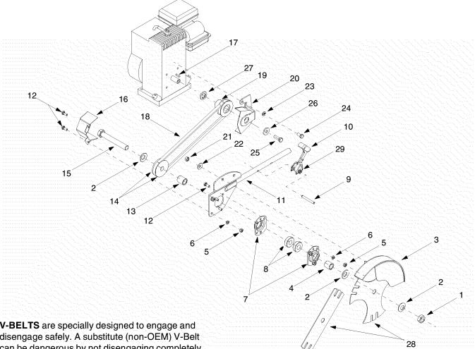
**V-BELTS** are specially designed to engage and disengage safely. A substitute (non-OEM) V-Belt can be dangerous by not disengaging completely.
