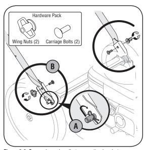
Figure 3-2: Secure lower handle to mounting brackets.
