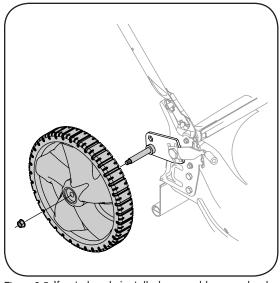
Figure 3-5: If not already installed, assemble rear wheels.
