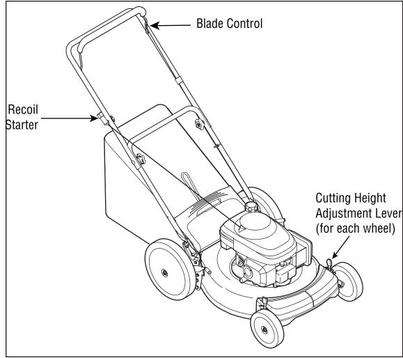
Figure 4-1: The main components on the mower.
