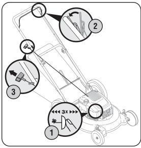
Figure 4-2: Starting the Briggs & Stratton/Tecumseh engine.
