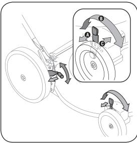
Figure 3-6: Use adjustment levers at each wheel to change the cutting height.
