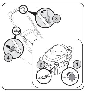
Figure 4-3: Starting the Honda engine.
