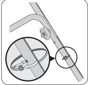
Figure 3-4: Secure cable to handle using cable ties.
