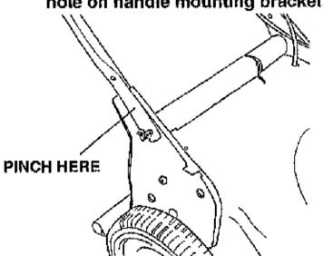
Step 7. Attach control cables to handle with pull ties found on the handle.
