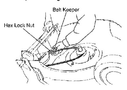
Mower shown tipped on engine for clarity. Remember, only tip mower back on its handle with the spark plug facing up. Otherwise, oil will spill if turned upside down.
