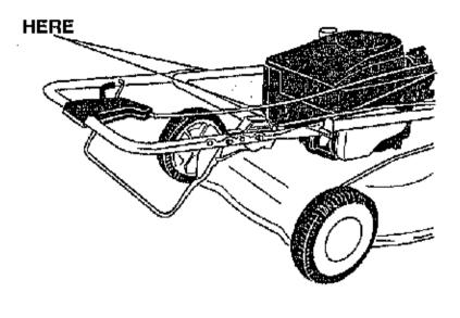
Step 4. Raise complete handle assembly until it clicks into place. Make sure not to kink the control cables.
