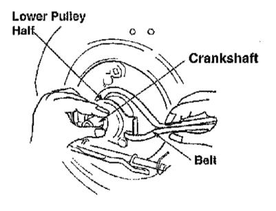
Step 20. Place belt between the two pulley halves on the crankshaft. Make sure to route the belt inside the belt guard pin.
