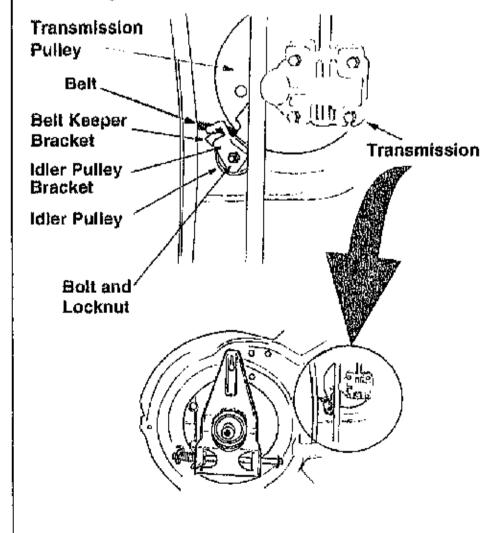
Step 18. Pivot the control arm down away from the pulley and belt.
