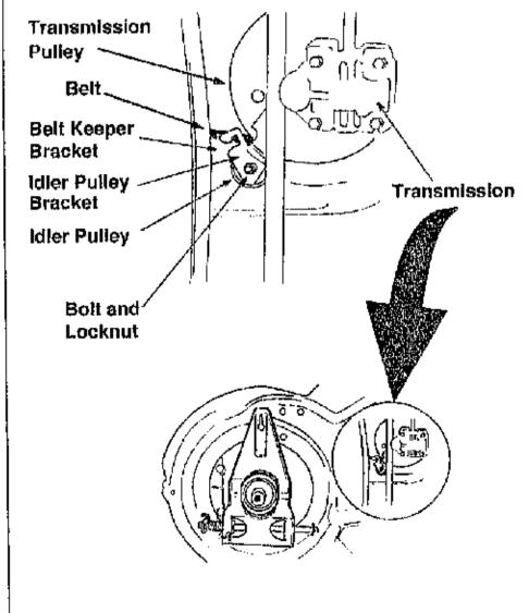
Step 13. Squeeze the belt together and push belt forward. Press the control arm inward towards the deck and remove the six speed cable from the slot.
