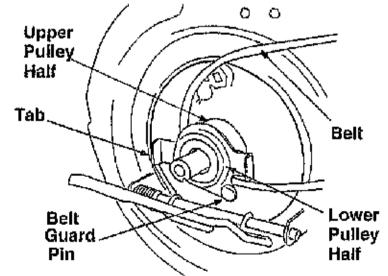
IMPORTANT: When changing the belt, do not disassemble the lower pulley assembly.
