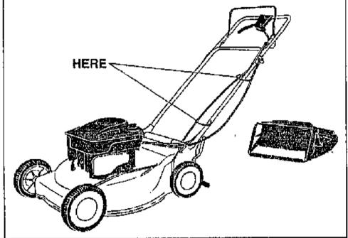
Step 8. Loosen the wing nut holding the rope guide to the upper handle.
