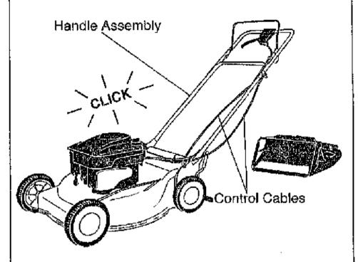
Step 5. Pinch lower handle against mounting bracket with pliers.
