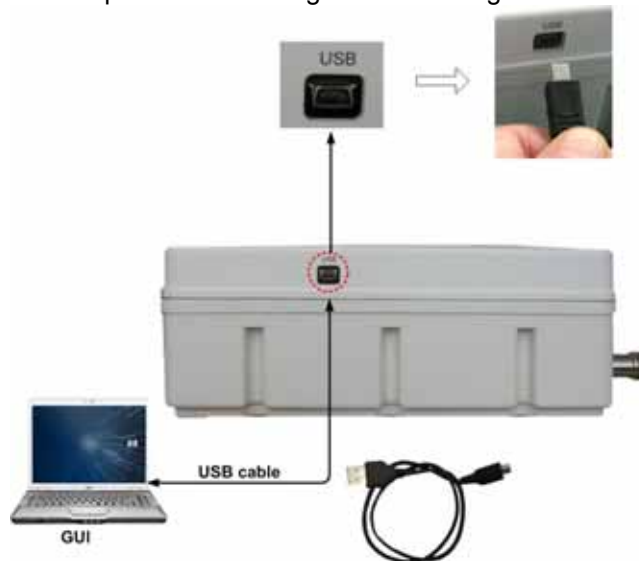
Figure 10 Connection of Laptop PC
