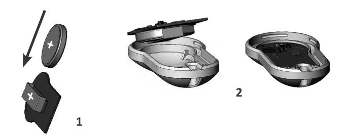
c. Reassemble the intermediate part and the push button and place over the electronic board.
