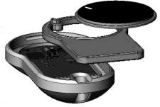
c. Take out the electronic board with the battery and remove battery.
