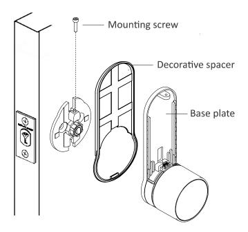
**Note:** In case the "Male rectangle" on the adapter is not aligned with the "Female rectangle" on the Knob, the unit will not engage properly and may cause to malfunction.
