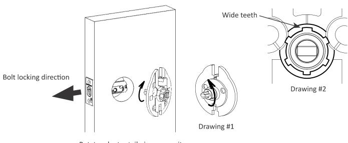
Rotate adapter tail piece opposite to the bolt locking direction
