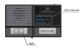
A 18650 Li-battery was included in this outdoor intercom. This intercom also can support AC adapter as power supply. Before to mount this outdoor intercom. We need to charge this intercom with 5V/1A AC adapter for 4-5 hours to make sure the Li-battery was full. When it charged, The Talking/ charging LED would light. When the Li-battery was full, the Talking/charging LED would turn off.
